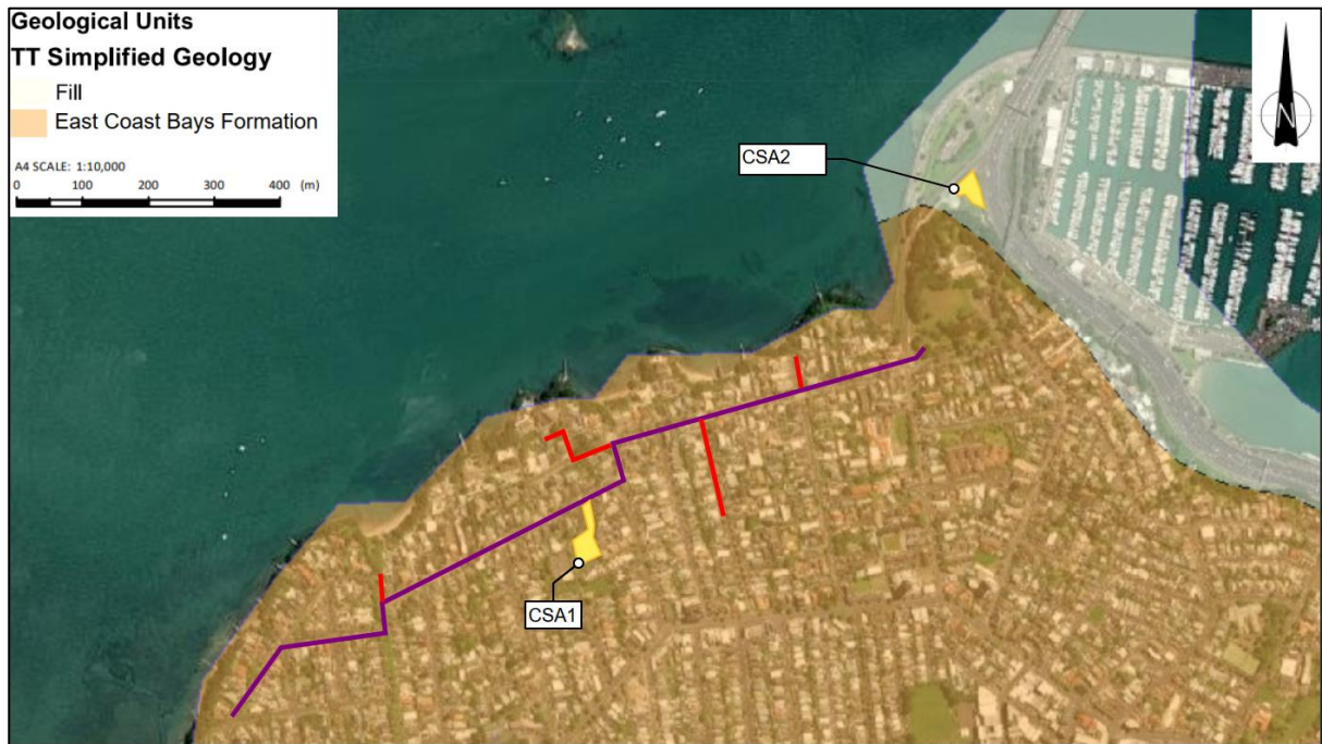
Figure 3.3: Published geology map of alignment, connecting pipes, CSA1 and CSA2 (source: Kermode).
