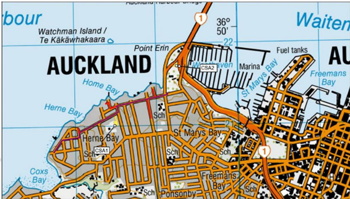
Figure 1.1: Approximate Herne Bay Tunnel alignment shown in purple, connecting pipes to engineered overflow points in red and CSAs shown in yellow (Source: Topomaps NZ)
